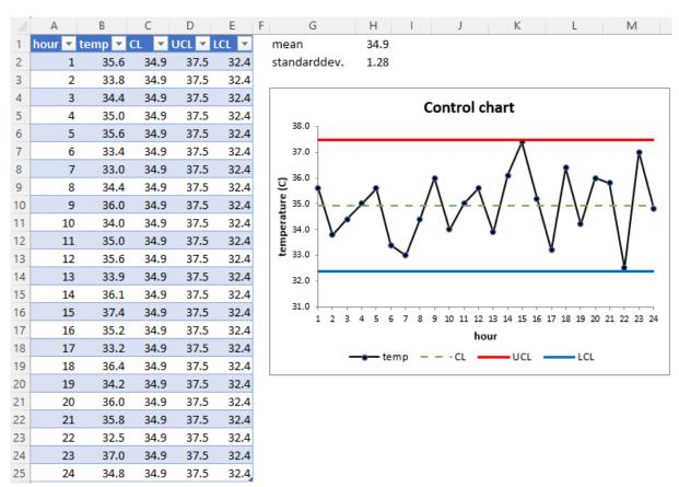
Figure 10.25: Control chart for the temperature in a chemical reactor.
